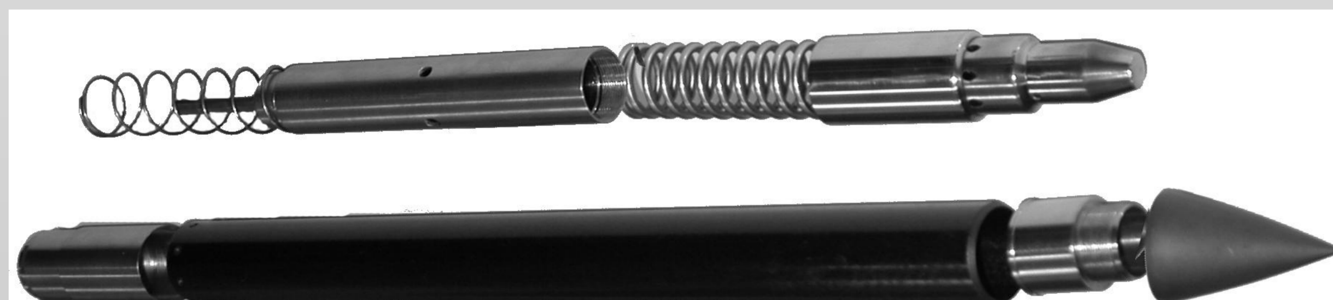
Fig. 2. The laboratory model of the mole penetrator: casing with the tip (bottom) and the hammer with the support (top)
